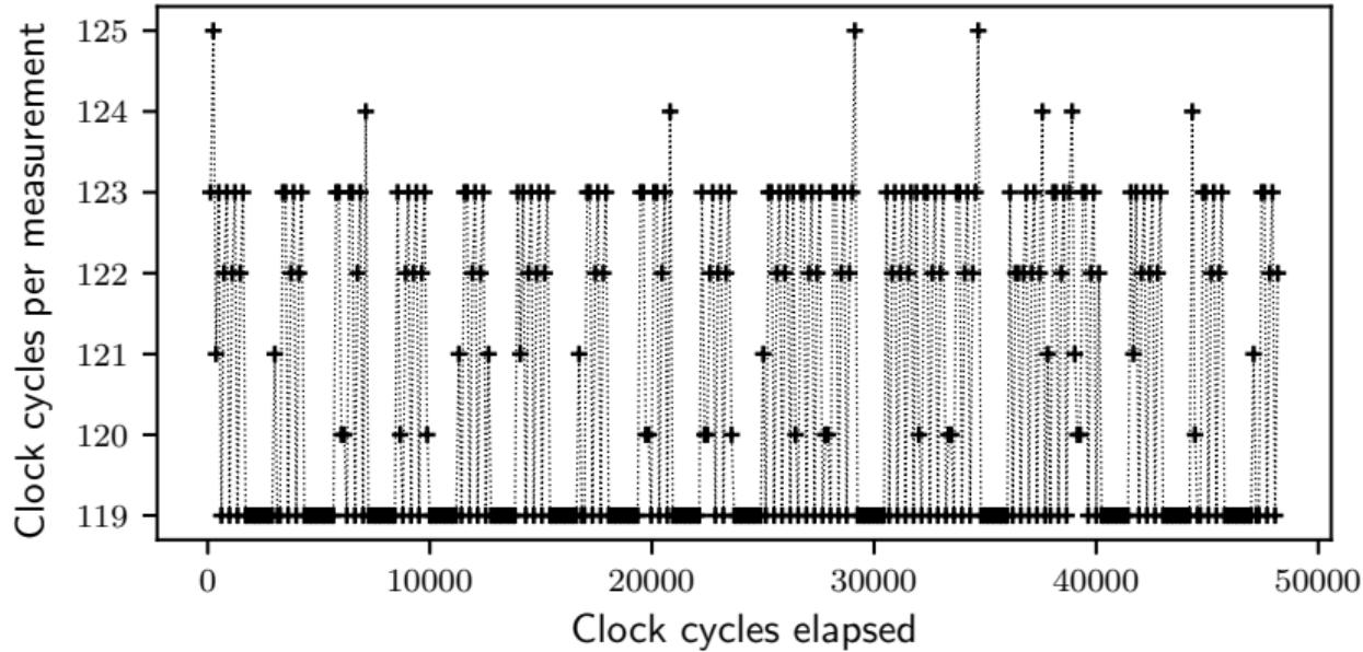
1 Mbit/s noise-based signal, pattern 010101010101010100010001000101010, 1 loop per measurement
