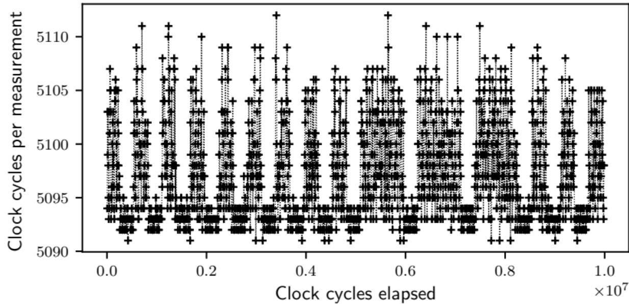
10 kbit/s noise-based signal, pattern 01010101010101010100010001000101010, 1000 loops
