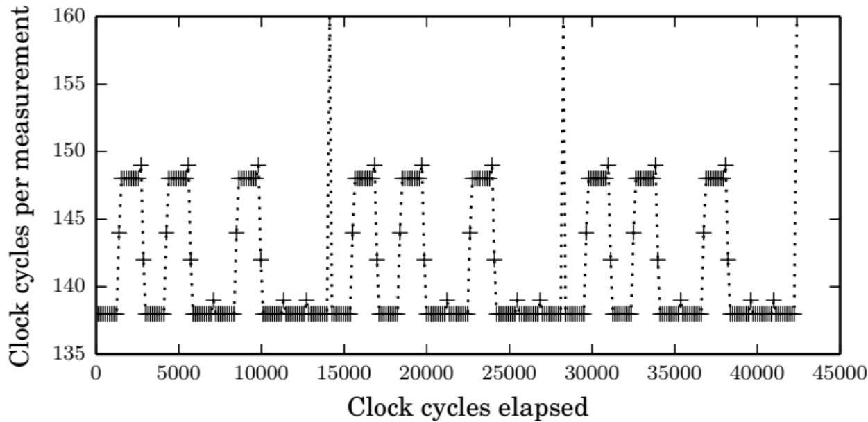
1 Mbit/s throughput-based signal, pattern 0101001000, 12 loops per measurement
